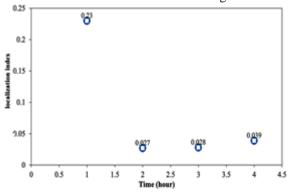
Fig. 3: Localisation index (LI) values of the HSLA base metal/ WM pair calculated for each hour of the ZRA test at ambient temperature.
