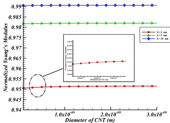
Figure 3. Diameter dependent Young modulus of carbon nanotube for constant lengths
