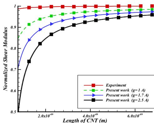
Figure 4. Size dependent shear modulus of carbon nanotube.
