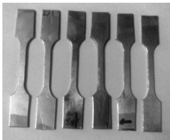
Figure 1. Standard specimens for uni-axial test
