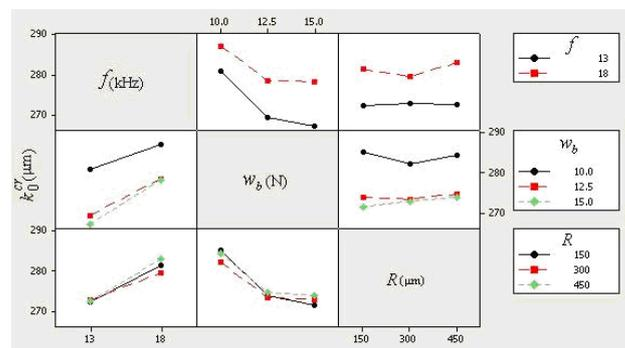
**Figure 2. Effects of the discharge frequency, wire tension and the curvature radius on curved slot width ( $k_0^{cr}$ )**
