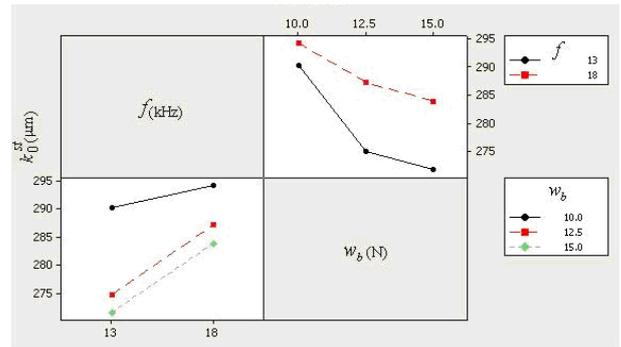
**Figure 1. Effects of the discharge frequency and wire tension on the straight slot width ( $k_0^{st}$ )**
