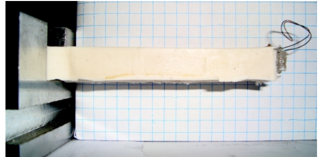
Figure 4. Shape memory beam (experimental method) is increased, as temperature in the shape memory wire increased. If input current is controlled, beam deformation will be controlled too. So, fiber's temperature is proportional to the input current. According to the experimental results and theoretical analysis, it can be concluded that to probe large flexural deformation, selection of elastomer field with shape memory fibers is an appropriate idea.
