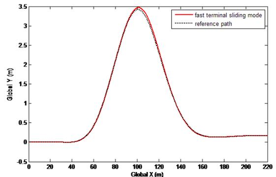
**Figure 2. Lateral position in double lane change maneuver under road disturbance and mass uncertainty**
