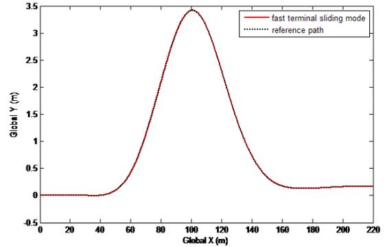
**Figure 1. Lateral position in double lane change maneuver**
