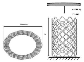
Figure 5. Boundary condition and loading
