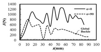
Figure 3. Force-displacement curve for tubes with cell angle  $\alpha$ =0 and  $\alpha$ =90
