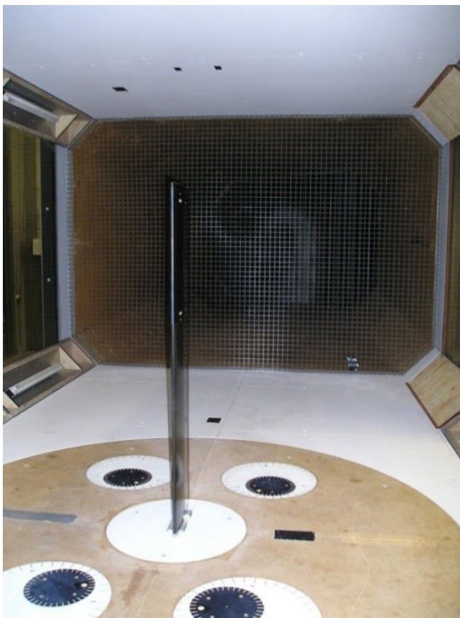
Figure 2. Installed model in the wind tunnel test section
