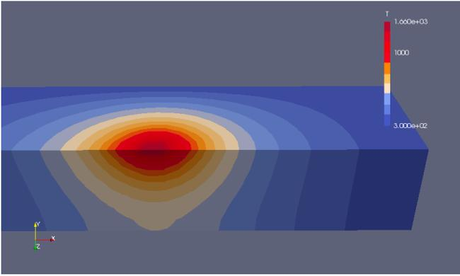
Figure 1. Three-dimensional temperature distribution in depth direction of part after 1 s
