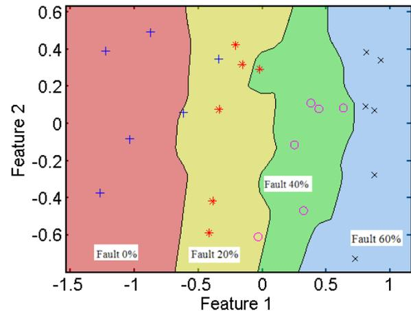
Figure 3. Classifier results for faulty gear wear
