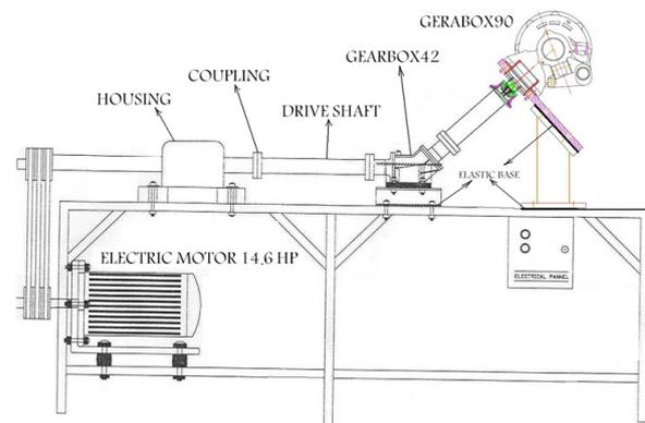
Figure 1. Schematic illustration of the experimental setup
