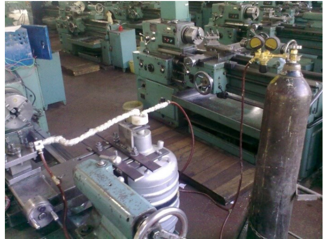
Fig. 1. Cryogenic cooling system
