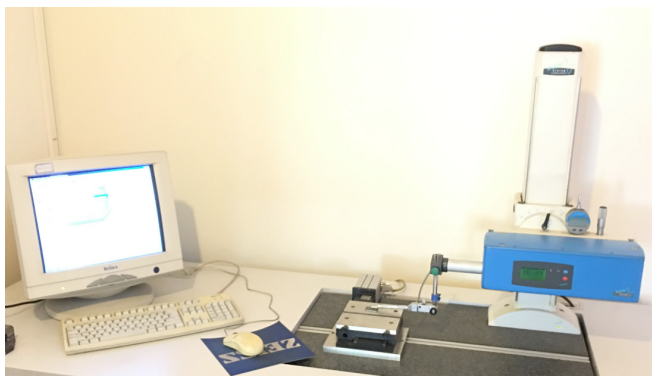
Fig. 2. Roughness measurement of Samples
