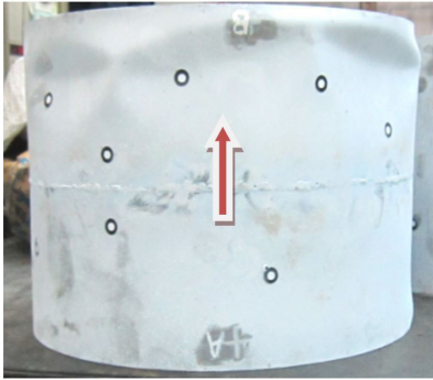
Fig. 21. Buckling deformation of the shell specimen SLC2
