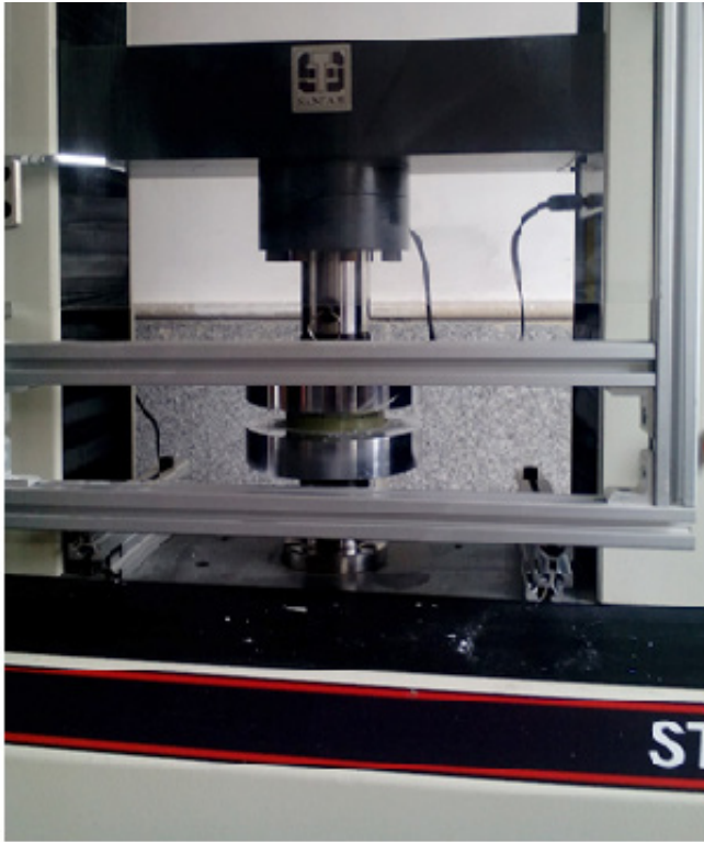
Fig. 16. Specimen and experimental set up of compression test
