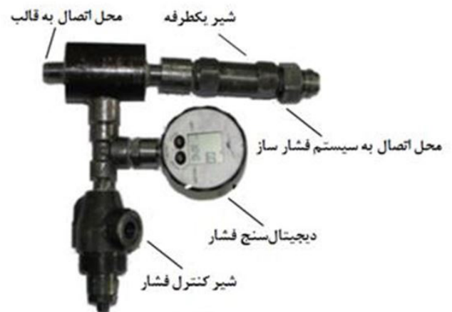
Fig. 5. Pressure control system
