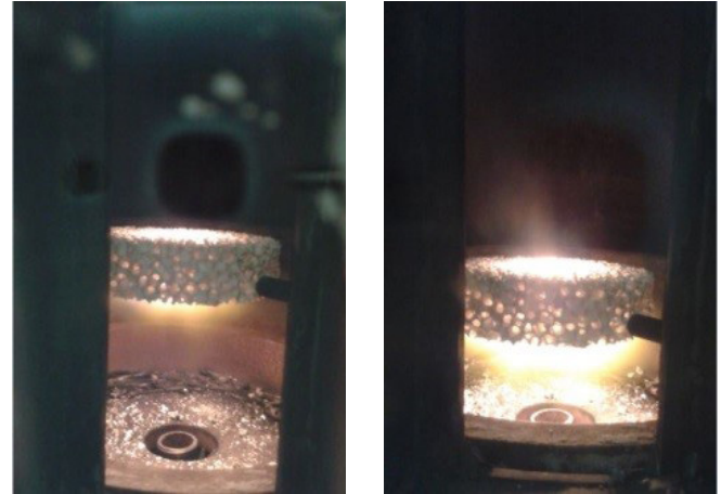
Fig. 11. Flames establishment at \phi=0.82 for burner by \epsilon=10 and (a) h=5 cm (b) h=8 cm
