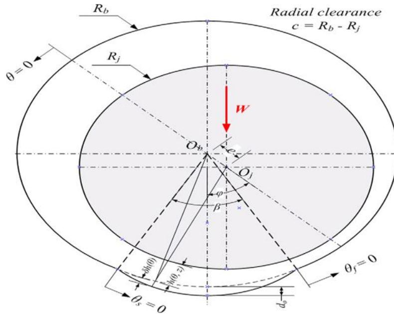
Fig. 1. Journal bearings geometry by considering abrasion
