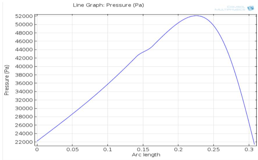
Fig. 2. Pressure at various arcs length with abrasion at  $\varphi=90^\circ$
