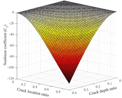
Fig. 2. Changes in the nonlinear coefficient ( $C_2$ ) for different crack depth and location ratios
