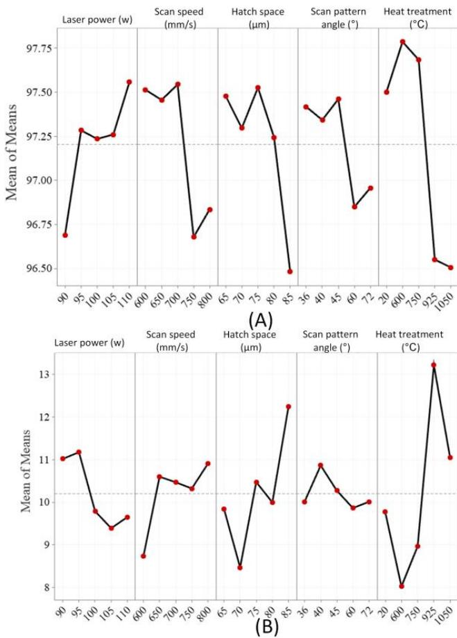
Fig. 1. Taguchi Mean Analysis for optimization of (A) Relative density, and (B) Surface roughness, separately [5, 6]
