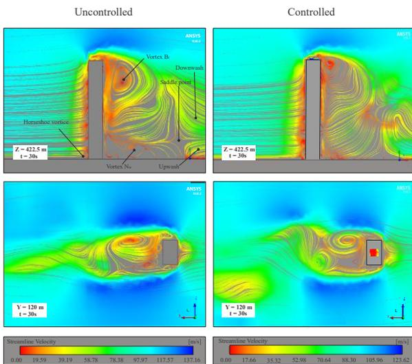
**Fig. 3. streamlines in plans of XY and XZ for controlled and uncontrolled modes**
