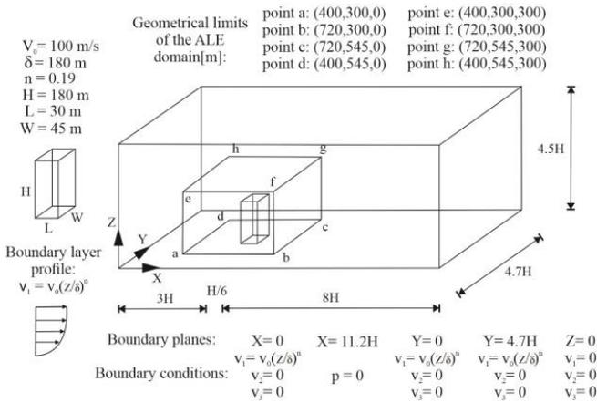
**Fig. 1. Geometrical characteristics and boundary conditions used in the aeroelastic analysis of a high-rise building model**
