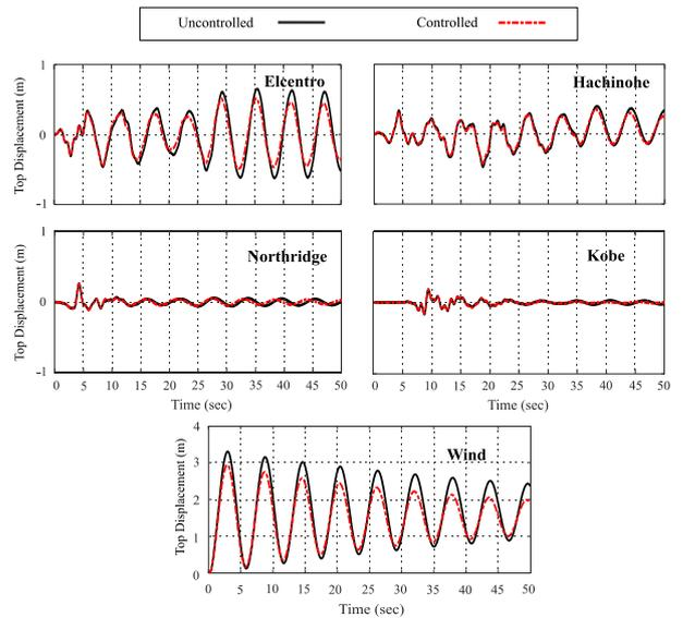
**Fig. 4. The top of structure Longitudinal displacement's time history under wind and four near and far-field records for controlled and uncontrolled modes**
