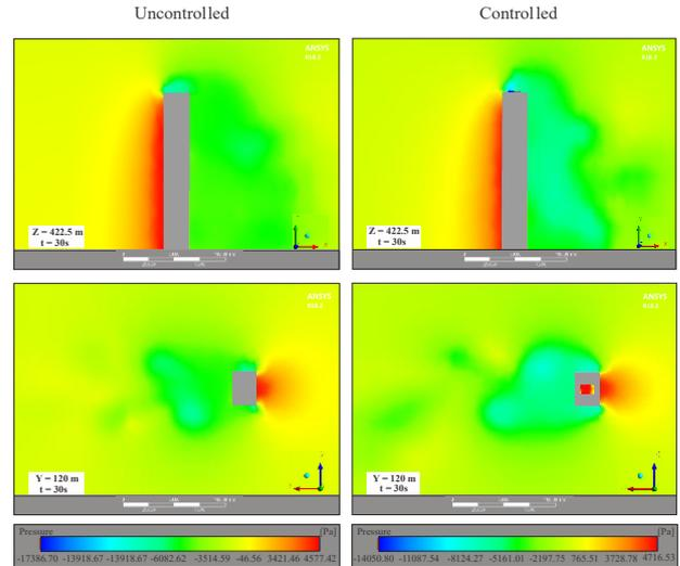
**Fig. 2. Distribution of pressure in plans of XY and XZ for controlled and uncontrolled modes**
