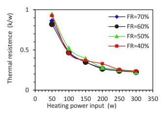
Fig. 1. Thermal resistance vs input heating power for various filling ratios in the vertical position
