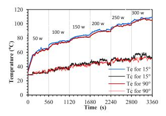
Fig. 3. Comparison of the transient evaporator and condenser temperature in inclination angle 15 and 90 degrees
