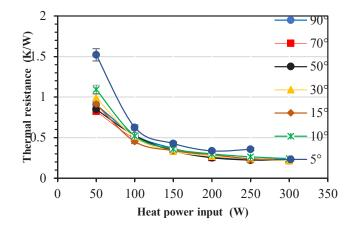
Fig. 2. Thermal resistance vs input heating power for various inclination angles of PHP
