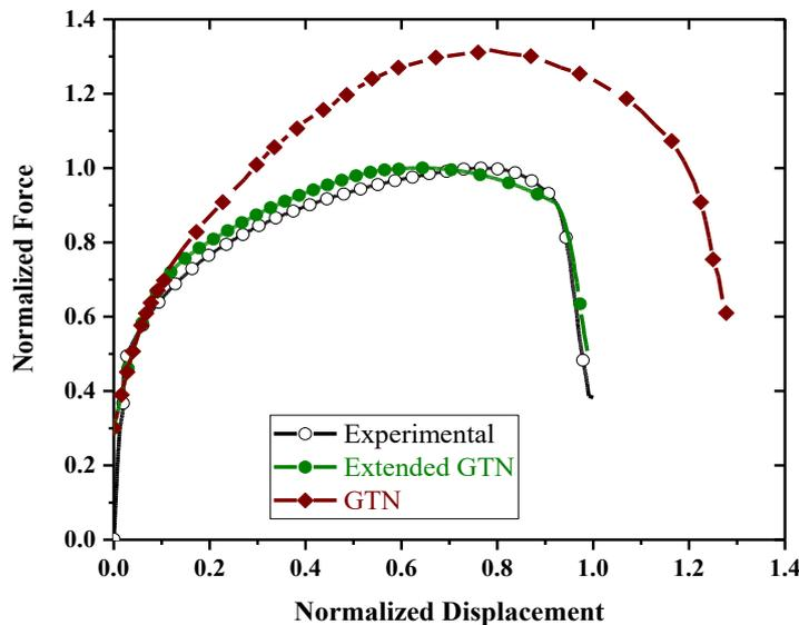
Fig. 1. Experimental and numerical force-displacement curves for shear specimen
