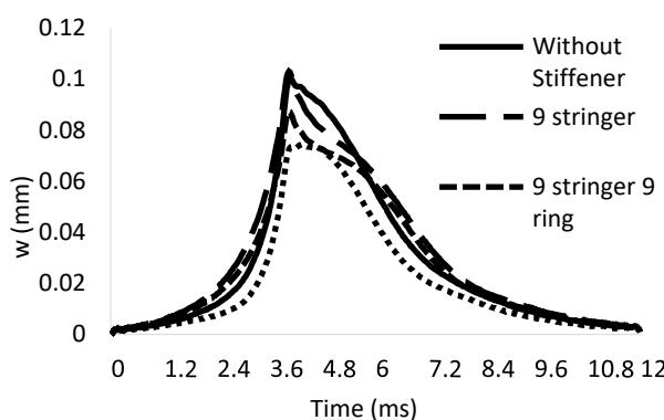
**Fig. 4. Analysis of the effect of different types of stiffener on the radial convection of the cylindrical shell**
