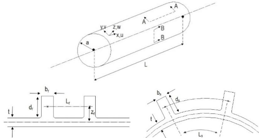
**Fig. 1. The geometry of shell and stiffeners**
