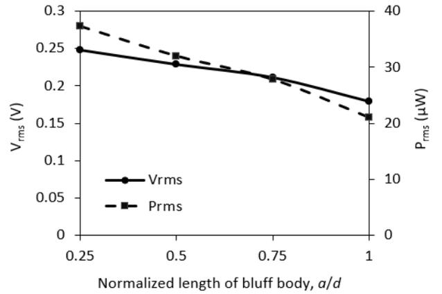
**Fig. 2. Effect of the length to height ratio on the harvester performance**
