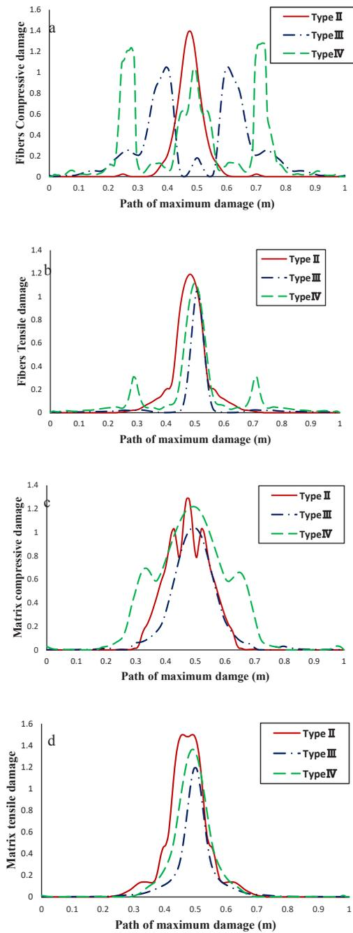
**Fig. 3. The amounts of damage to the composite for the first case: a) fibers compressive damage, b) fibers tensile damage c) matrix compressive damage, d) matrix tensile damage**
