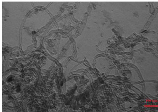
**Fig. 2. TEM image of the synthesized CNT**
