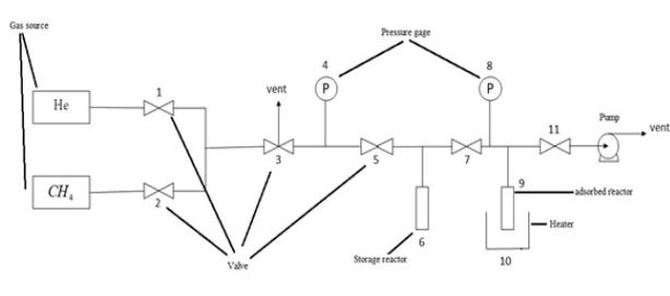
Fig. 1. the schematic of the methane adsorption apparatus
