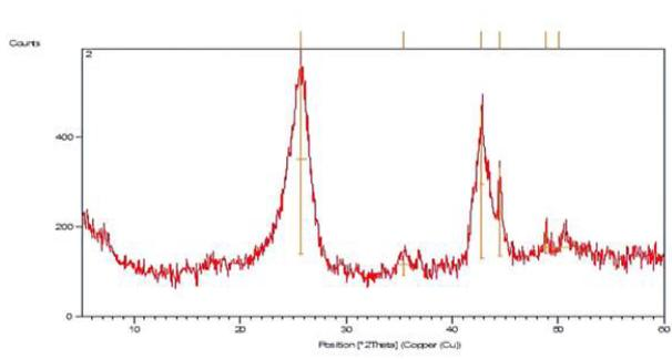
Fig. 3. XRD pattern of the carbonous adsorbent
