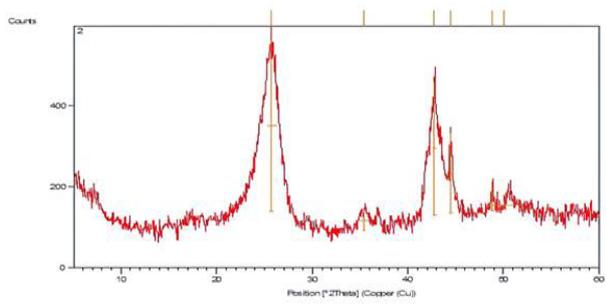
**Fig. 3. XRD pattern of the carbonous adsorbent**
