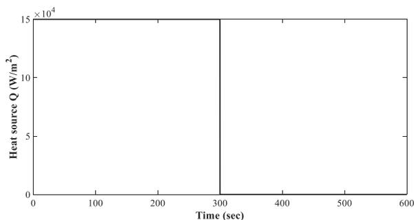
Fig. 2. Heat flux used for calculating desired thermal dose
