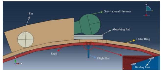
Fig. 2. The finite element model of the problem
