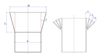
Fig. 1. Schematic of tube end flaring
