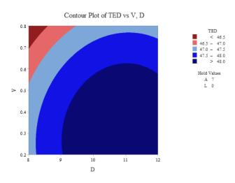
Fig. 3. Effect of tool diameter and tool vertical step
