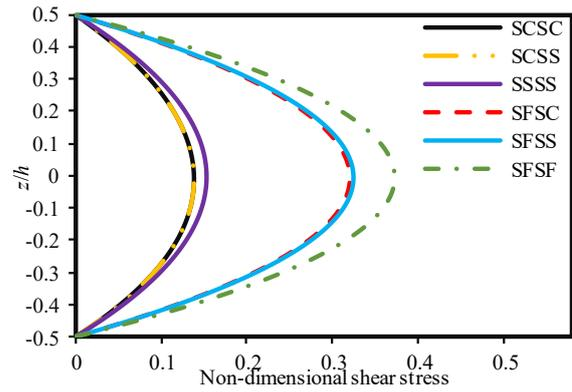
**Fig. 3.** Variation of non-dimensional transverse shear stress through the smart FG plate thickness (n=2, a/h=5).
