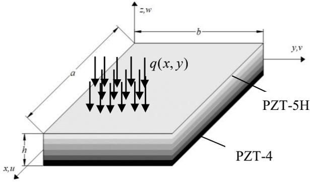
**Fig. 1. Geometry of functionally graded piezoelectric plate**
