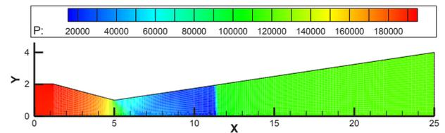
Fig. 7. Pressure contour in the 2-D nozzle
