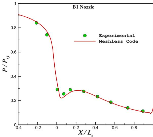
Fig. 3. Nondimension pressure distribution over nozzle B1 wall
