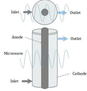
Figure 1. Schematic diagram of EMER
