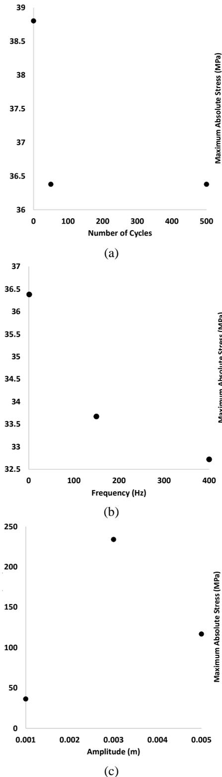
Fig. 3 Maximum absolute value of the residual stress calculated along the y-axis on the cross-section for (a)  $\delta = 1\text{mm}, f = 1\text{Hz}$ ; (b)  $\delta = 1\text{mm}, n = 10$ ; (c)  $f = 1\text{Hz}, n = 10$
