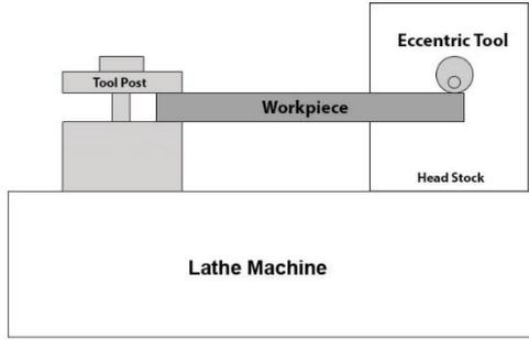
Fig. 1 Proposed vibrational stress relief configuration
