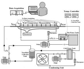
Fig. 1. Schematic diagram of the experimental apparatus.
