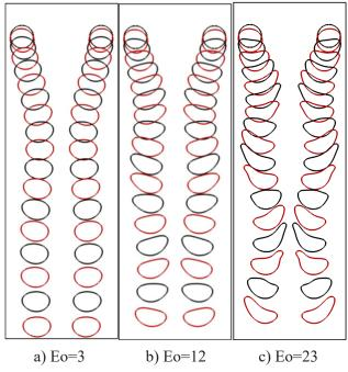
Figure 1. Falling two adjacent droplets by different initial lateral positions from near the side walls  $(Oh=0.072, t_a^*=0, \Delta t^*=1)$
