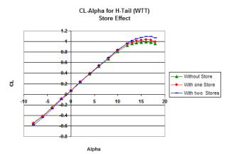
Figure 2.  $C_1 - \alpha$  with and without external tank
