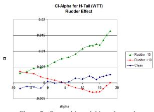
Figure 7.  $C_i - \alpha$  with variable ruder angle
