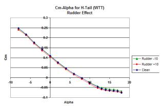
Figure 6.  $C_m - \alpha$  with variable ruder angle
