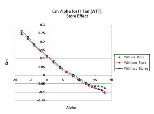
Figure 4.  $C_m - \alpha$  with and without external tank
