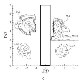
Figure 1. Tip vortices and base vortices in  $\omega_x$  contours (a) X/D=5 (b) X/D=7.5 (c) X/D=10; vorticity contour increment 0.05, minimum vorticity contour -0.4 and maximum vorticity contour + 0.4
