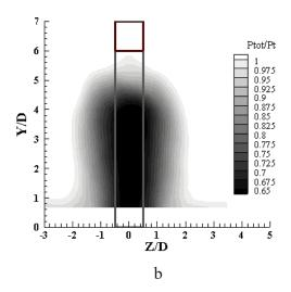
Figure 2. Non-dimensional total pressure at *X/D*=5: (a) flat free end; (b) elliptical free end
