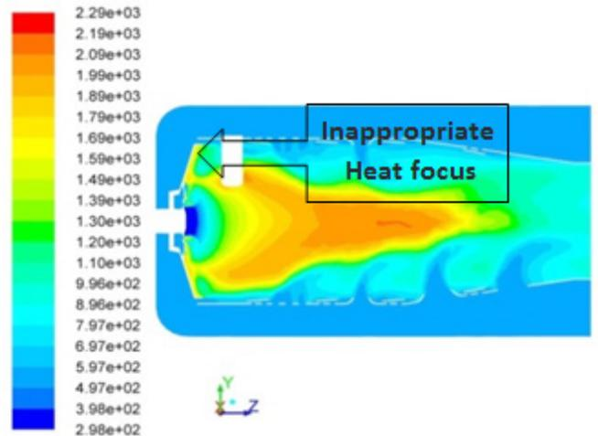
Figure 2. Temperature profile in combustion chamber
