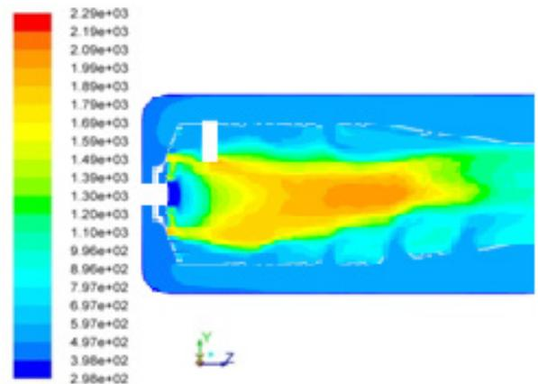
Figure 5. Temperature profile in optimized combustion chamber
