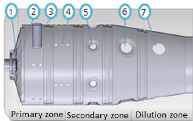
Figure 1. Combustion chamber geometry
