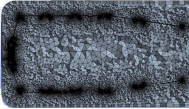
Figure 2. Mesh geometry of combustion chamber
