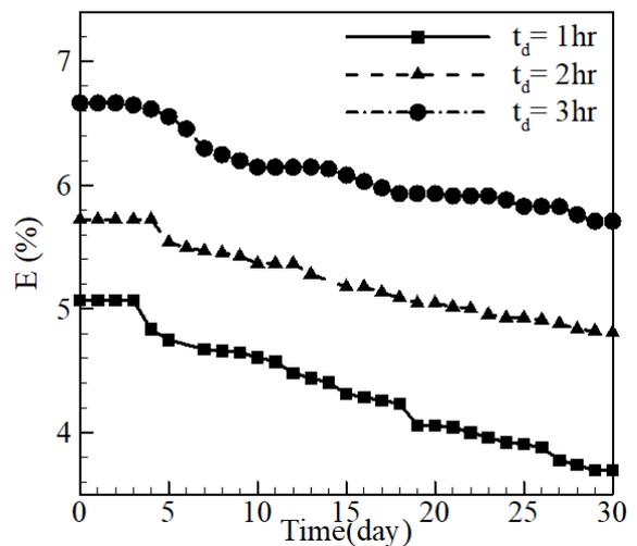
Figure 2. The heat transfer enhancement ( $E$ ) over a period of 30 days for  $Ra=10^2$  and  $\phi_b=0.013$ .
