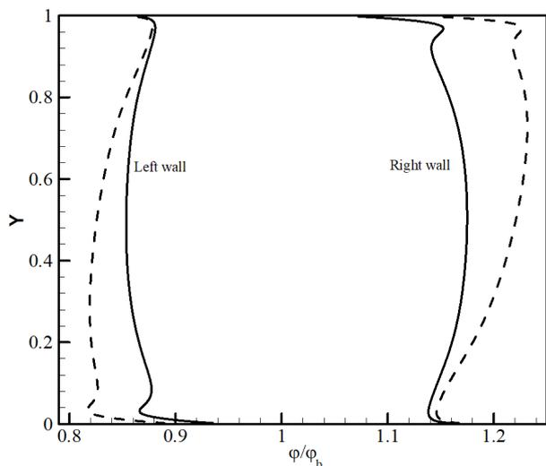
**Figure 2. Distribution of volume fraction of nanoparticles near the walls without sedimentation velocity (—) and with it (-----)**
