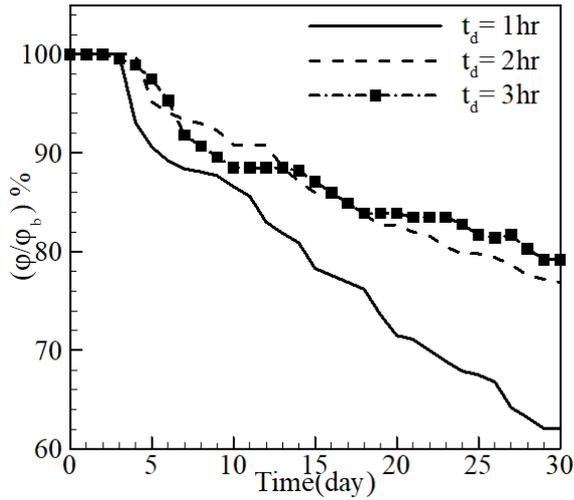
Figure 1. The rate of sedimentation nanoparticles for water- $\text{Al}_2\text{O}_3$  nanofluid and  $\phi_b=0.013$  [2]
