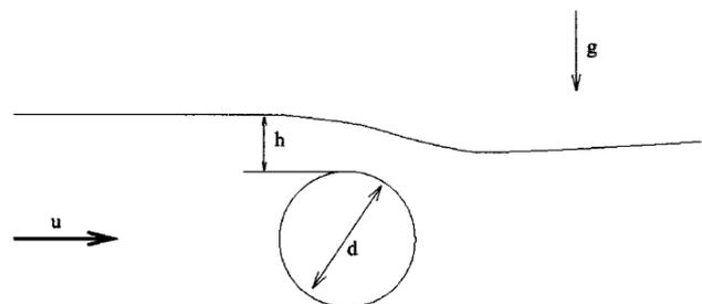
Figure 1. Flow around a circular cylinder near the free surface of fluid
