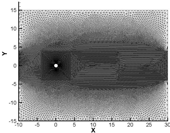
Figure 2. Numerical grid (dimensions in meter)
