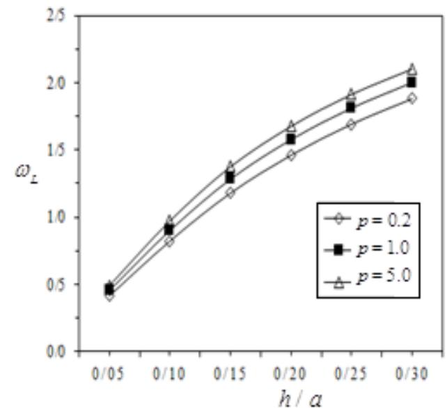
**Figure 1. Effect of thickness to dimension of a MEE square**
