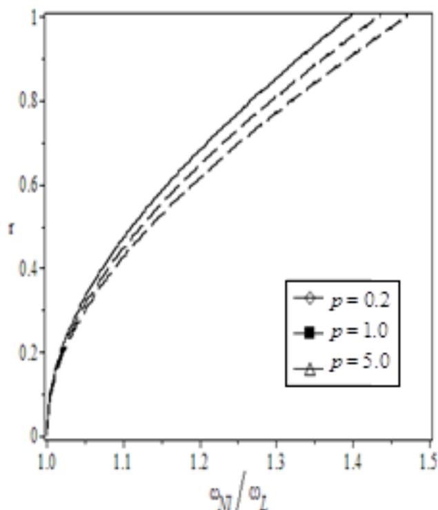
Figure 2. Effect of coefficient of power law number  $p$  on the ratio of nonlinear to linear natural frequency
