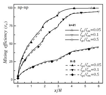
Figure 2. Mixing efficiency value of Nernst-Planck model and H-S model for *K*=41
