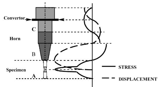
Fig. 1. Displacement and stress distribution [1]
