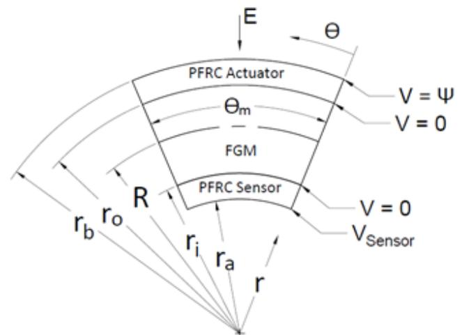
Figure 1. Problem geometry parameters and applied electric voltage location
