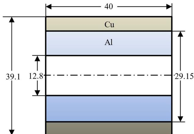
Figure 1. Configuration of the bimetal tube before extrusion (dimension are in mm)
