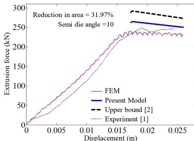
Figure 2. Comparison of analytical model, FEM, experimental and the upper bound solution [2] force-displacement curves
