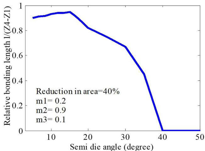
Figure 3. Effect of semi die angle upon the bonding length at the interface between layers
