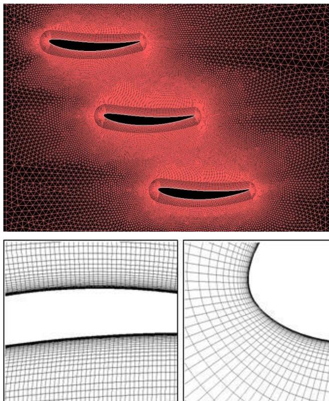
Figure 2. Grid domain near the blade surfaces
