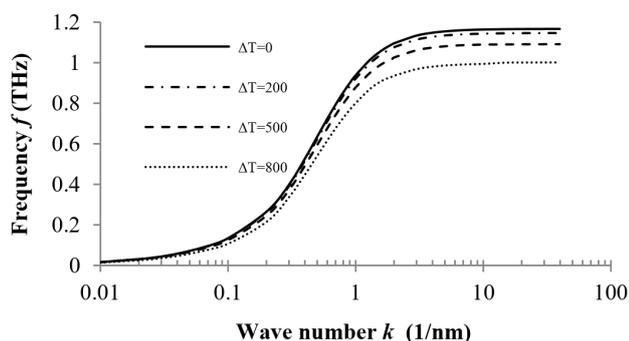
Fig. 1. Effect of various temperature changes on the wave frequency of FG nanoplates ( $p=1, \mu=1 \text{ nm}^2$ ).
