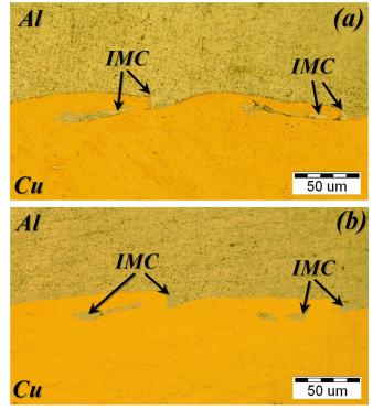
Fig. 2. Cross-section optical image of Al/Cu interface with wavy structure and minimum intermetallic compounds (a) after explosive welding process (b) after the last stage of shape rolling process.
