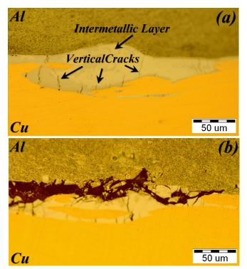
Fig. 1. Cross-section optical image of Al/Cu interface with thick and continuous intermetallic layer (a) after explosive welding process (b) after the last stage of shape rolling process.
