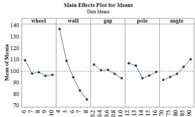
**Fig. 2. The effect of geometric parameters on mean magnetic flux density**
