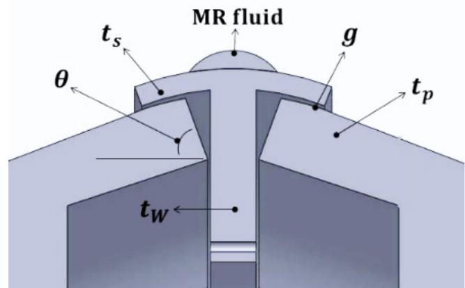
**Fig. 1. Effective geometric parameters on magnetic flux density in the material removal region**
