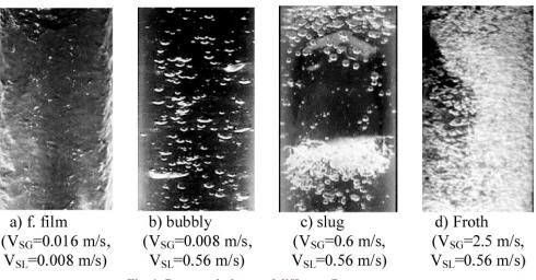
Fig. 1. Processed photos of different flow patterns
