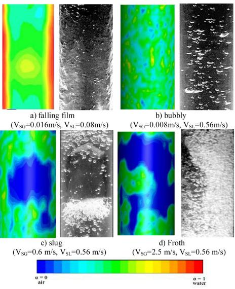
Fig. 2. Contours of phase 2 (air) volume fraction and comparison with experimental results
